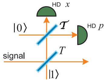
Figure 4.6: Scheme for realizing the  $X$ -gate.  $T$  and  $\mathcal{T}$  denote transmissivities of the respective beam splitters. HD - homodyne detectors.
