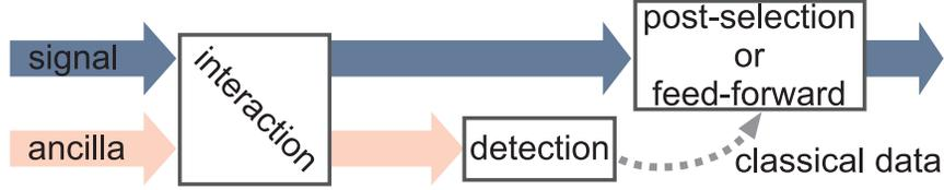
Figure 2.1: Conceptual description of a measurement induced operation.
