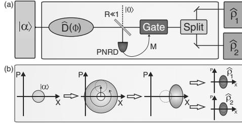
FIG. 1. (Color online) (a) Schematic of the cloning scheme. Two identical clones  $\hat{\rho}_{1,2}$  are created by probabilistic amplification and subsequent symmetric splitting. (b) Evolution of a coherent state in phase space during the cloning process.
