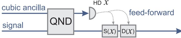
Figure 5.1: Scheme for deterministic implementation of the nonlinear cubic gate. QND - quantum non-demolition interaction, HD - homodyne detector,  $S(x)$  and  $D(x)$  represent the squeezing and displacement, respectively, driven by the measured value  $x$ .
