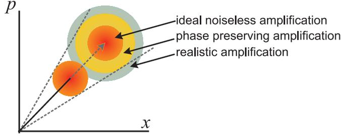
Figure 3.1: Illustration of amplification for coherent states of light. The circles schematically demonstrate profile of the states' Wigner functions in phase space.
