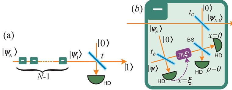
Figure 4.5: (a) Scheme for generating a single photon state from an arbitrary state with finite dimension. (b) Detailed scheme for a single subtraction step.  $t$ ,  $t_a$ , and  $t_b$  denote transmission coefficients of the respective beam splitters, BS - balanced beam splitter, HD - homodyne detection,  $D(\xi)$  - displacement driven by the measured value  $\xi$ .
