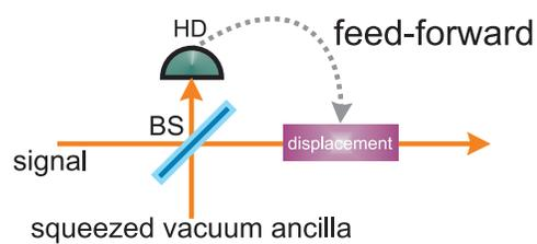
Figure 2.3: Measurement induced realization of the squeezing operation. BS - beam splitter, HD - homodyne detection
