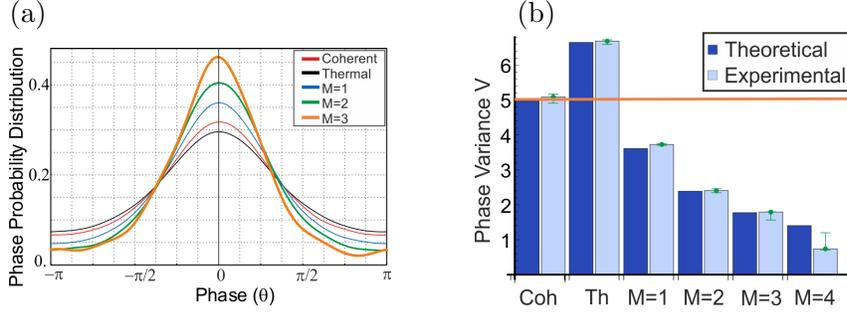
Figure 3.3: (a) Phase distributions for the initial coherent state and different levels of amplification. (b) Phase variances for different levels of amplification. Experimental data of [A2].
