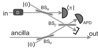
FIG. 4. (Color online) Schematic representation of the approximate single-mode Hadamard gate.  $BS_u$  stands for a highly unbalanced weakly reflecting beam splitter, while  $BS_r$  is a beam splitter with transmission coefficient  $t_r$  used to set the parameter  $\Gamma$ . APD stands for an avalanche photodiode and  $\langle\pi|$  represents the suitable projective measurement (see text).
