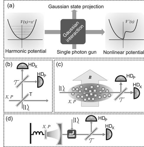
FIG. 1. (Color online) (a) Concept of the implementation of a nonlinear potential by single-photon guns, (b)  $X$  gate for a single mode of light using BS-type coupling, (c)  $X$  gate for a collective spin of cloud of atoms in magnetic field, and (d)  $X$  gate for the vibration mode of a mechanical oscillator.
