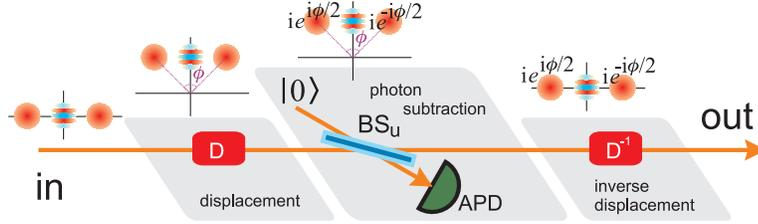
Figure 4.1: (Color online) Schematic representation of the single-mode phase gate. BS stands for a mostly transmitting strongly unbalanced beam splitter, APD stands for avalanche photodiode, and D represents the displacement operation.
