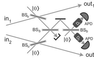
FIG. 3. (Color online) Alternative architecture of the two-mode controlled PHASE gate.  $\text{BS}_b$  stands for a balanced beam splitter, while  $\text{BS}_u$  represents a strongly unbalanced weakly reflective one. APD represents avalanche photodiode and  $D_1$  and  $D_2$  are the displacement operations. Numbers 1 and 2 distinguish the two participating modes, while labels “in” and “out” describe the input and output states of the gate.
