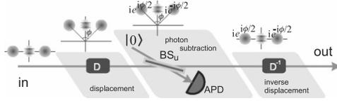
FIG. 1. (Color online) Schematic representation of the single-mode PHASE gate. BS stands for a mostly transmitting strongly unbalanced beam splitter, APD stands for avalanche photodiode, and  $D$  represents the displacement operation.
