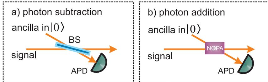
Figure 2.2: Schematic depiction of probabilistic implementation of photon subtraction (a) and photon addition (b). BS - beam splitter, NOPA - non-degenerate optical parametric amplifier, APD - avalanche photo diode.
