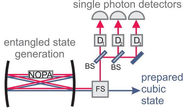
Figure 5.2: Scheme for probabilistic generation of a specific non-Gaussian state. The entangled two-mode squeezed state is generated in oscillator cavity with nonlinear medium (NOPA). The two frequency modes are separated by the frequency separator (FS) and one of the modes is divided on a sequence of beam splitters (BS), subject to suitable displacements  $D_1$ ,  $D_2$ , and  $D_3$ , and measured by single photon detectors.
