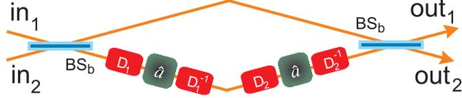
Figure 4.2: (Color online) Schematic representation of the two-mode controlled phase gate.  $\text{BS}_b$  stands for a balanced beam splitter and  $D_{1,2}$  represent displacements by  $\gamma_{1,2}/\sqrt{2}$ . Numbers 1 and 2 distinguish the two participating modes, while labels ‘in’ and ‘out’ describe the input and output state of the gate.
