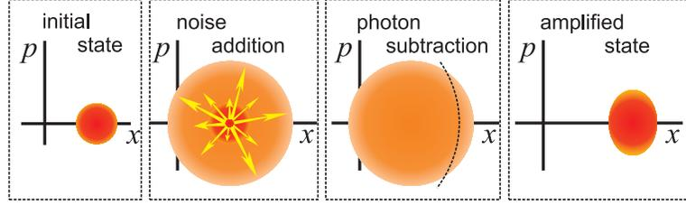
Figure 3.2: Phase space illustration of the noise powered amplification of a coherent state of light
