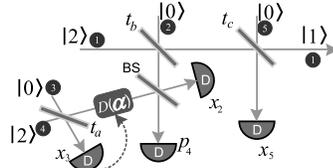
FIG. 3. (Color online) Complete setup for generation of a single-photon state from a pair of two-photon states.  $t_a$ ,  $t_b$ , and  $t_c$  denote transmittances of the respective beam splitters, while BS stands for a balanced beam splitter. Numbers 1–5 are used to label the modes involved.
