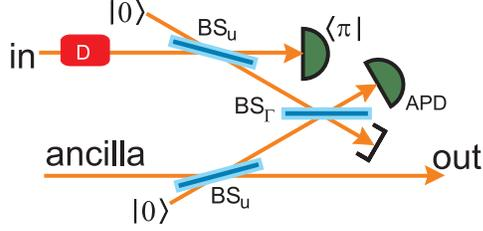
Figure 4.3: (Color online) Schematic representation of the approximate single-mode Hadamard gate.  $BS_u$  stands for a highly unbalanced weakly reflecting beam splitter, while  $BS_\Gamma$  is a beam splitter with transmission coefficient  $t_\Gamma$  used to set the parameter  $\Gamma$ . APD stands for a avalanche photodiode and  $\langle \pi |$  represents the suitable projective measurement (see text).
