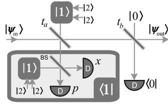
FIG. 5. (Color online) Complete setup for implementation of the nonlinear sign gate using only Gaussian operations and two-photon states as a resource.  $t_a$  and  $t_b$  transmittances of the respective beam splitters, while BS stands for a balanced beam splitter.
