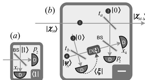
FIG. 1. (Color online) (a) Setup for projective measurement on a single-photon state. D—Homodyne detectors, BS—balanced beam splitter. (b) Setup for approximate photon subtraction. D—homodyne detector, BS—balanced beam splitter,  $t_{a,b}$ —beam splitter with transmittance  $t_{a,b}$ ,  $D(\xi)$ —displacement driven by detected value  $\xi$ .
