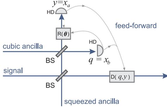
Figure 5.5: Scheme of the cubic gate realized by non-Gaussian adaptive measurement. BS - balanced beam splitter, HD - homodyne detection,  $R(\theta)$  - phase shift by angle  $\theta$ ,  $D(q, y)$  - displacement by value dependant of  $q$  and  $y$ .
