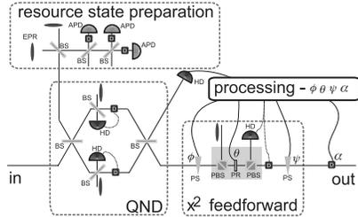
FIG. 2. (Color online) Schematic experimental setup of the deterministic  $x^3$  gate. BS, beam splitter; PBS, polarization beam splitter; PS, phase shift; PR, polarization rotator; APD, avalanche photodiode; HD, homodyne detection; and D, displacement.
