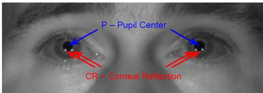
*Figure 7. Pupil centers and corneal reflections recorded by a Tobii Pro Spectrum 300 eye-tracker.*
