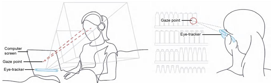
Figure 8. The principle of remote (left) and wearable (right) eye-trackers. Modified from Tobii.com.
