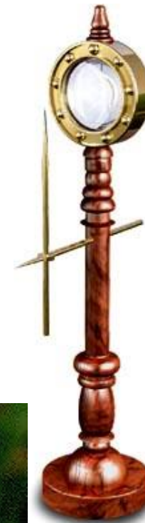
Simple Sliding Rod Microscope (circa 1640s)
