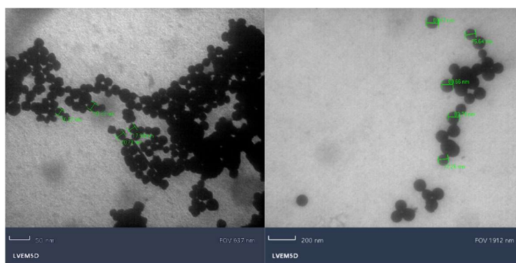
Nickel nanoparticles obtained by the solvothermal method
